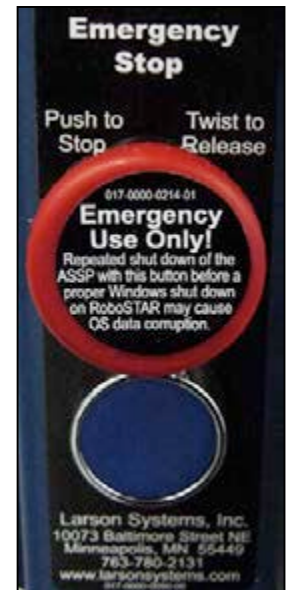
ASSP Control Panel Emergency Stop
