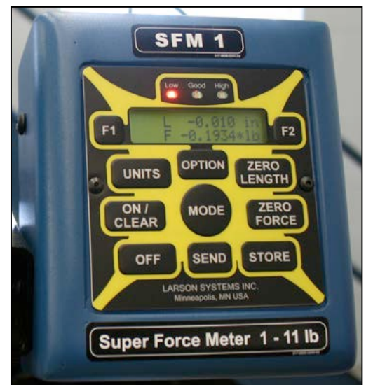
SFM – Load Station Control Panel
